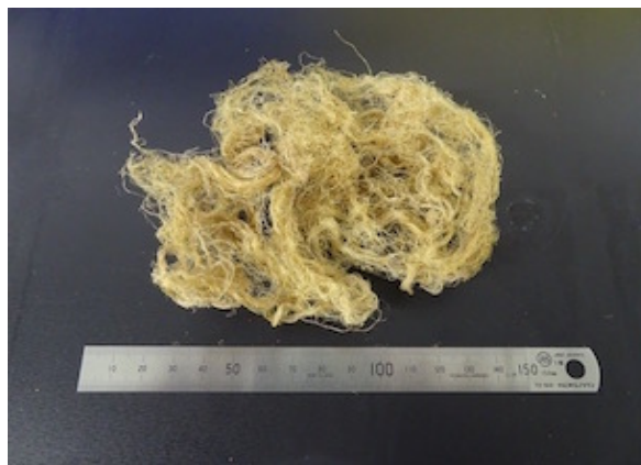
Figure 2. Alkali-treated banana fiber.
