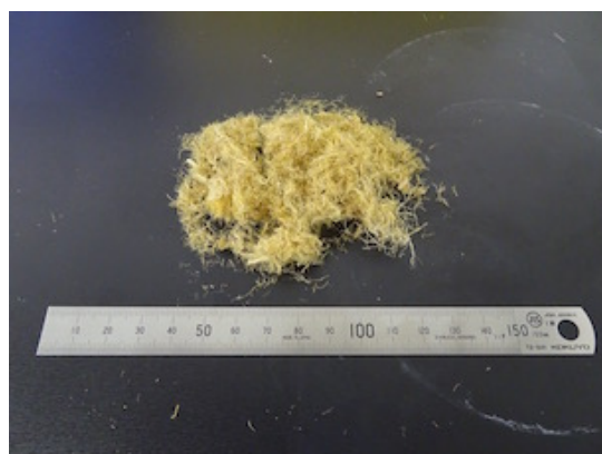
Figure 4. Alkali-treated banana fiber. The banana fiber was cut into the lengths of 5 mm.
