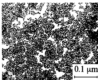
Figure 3. Transmission electron micrograph of zirconia from 0.36 kmol/m 3 Zr(IV), 1.03 kmol/m 3 free carboxylate solution at 200°C for 180 min.
