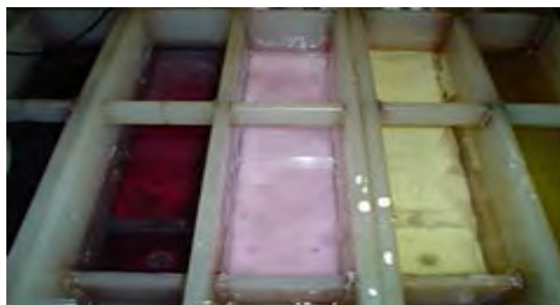
Figure 2 Settled gypsum precipitate in a D 2 EPHA strong acid strip circuit
