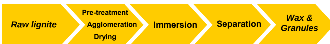
Figure 1. Schematically process design of the new immersion extraction of lignite
