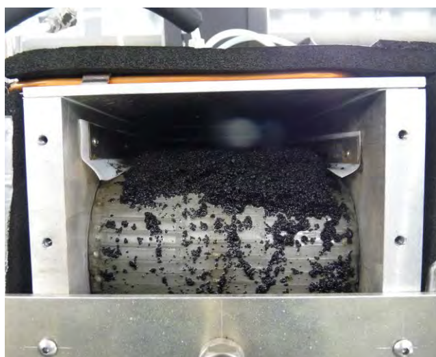
Figure 3. Illustration of the bulk flow at the drop-zone from the opened front side
