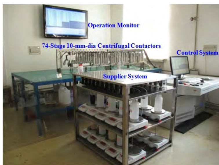
Figure 3 The demonstration test system
