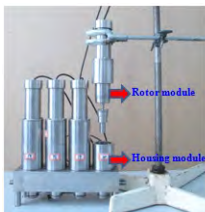
Figure 1 The \phi 10 mm annular centrifugal contactors.
