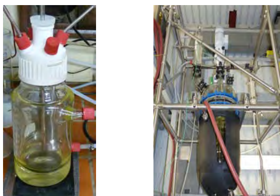
Figure 6. Photos of the two different used laboratory scales of immersion: 1L (left) and 50L (right)
