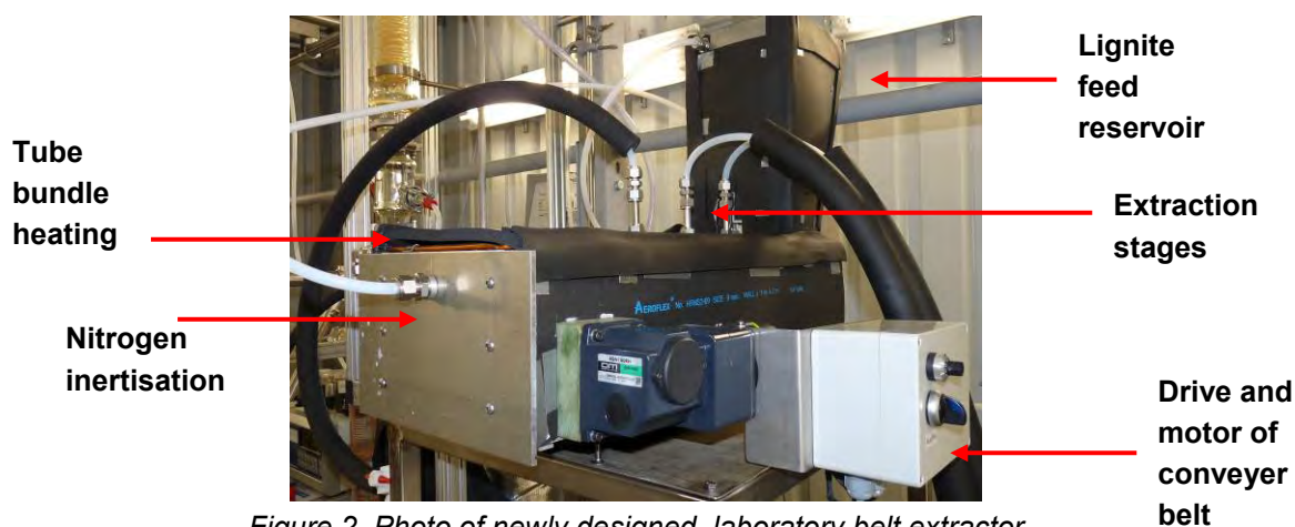
Figure 2. Photo of newly designed, laboratory belt extractor
